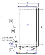
Drain Electrical inlet (power) RΩ Refrigerant Outlet
